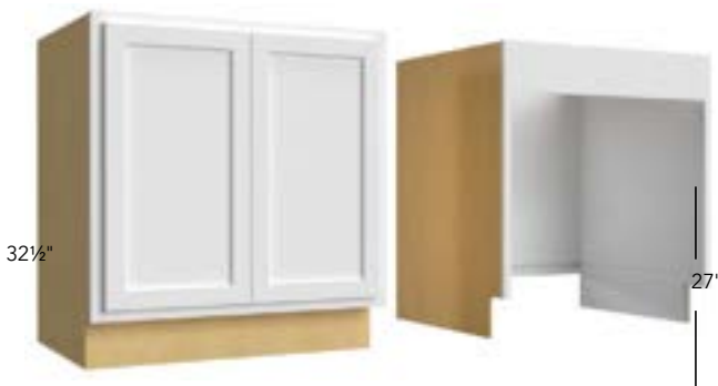
AFTER DOORS, FLOOR & TOE KICK ARE REMOVED
